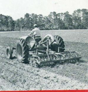
Flexible connections between gangs allow each gang to hug the contour of the ground. Allows uniform penetration on listed or uneven land.
