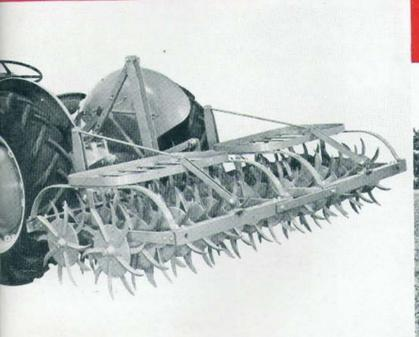
Tractor mounted, the Ferguson Rotary Hoe attaches in one minute by 3-point linkage of the Ferguson System. Raises and lowers by Finger Tip Control.
